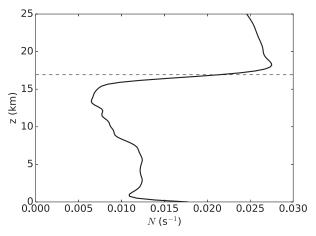
FIG. 2. Mean profile of the Brunt–Väisälä frequency N calculated from soundings taken every 3 h at the Darwin ARM site from 18 Jan to 3 Feb 2006. The dashed line denotes the cold-point tropopause at 16.9 km.
